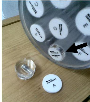
**Figure 3.** The lettered threaded caps and the orientation rails(arrow)
