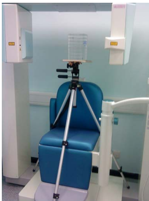
Figure 2. Equipment for active scatter measurements set up in CBCT facility
