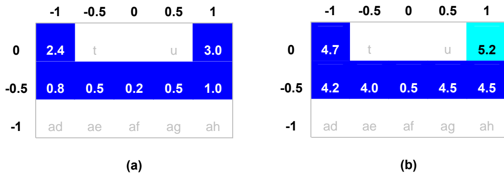
Figure 8. Comparison of scatter at 1 m (isocentre height) and 2 m from the ground at the rear and sides of the NewTom 9000
