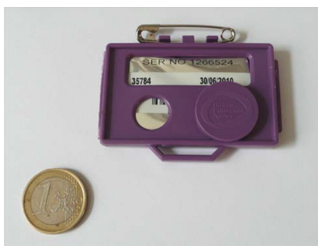
Figure 4. Personal dosimeter containing TLD used for passive measurement of scatter
